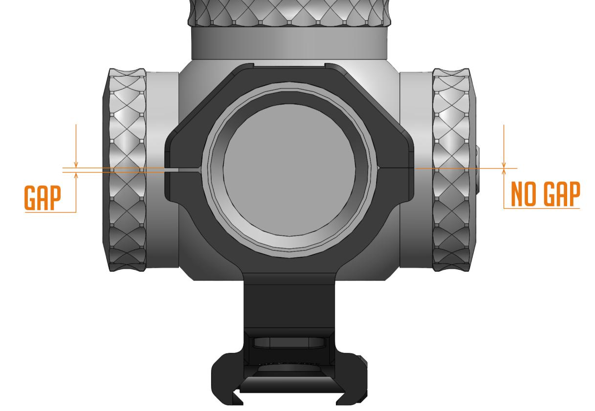
02. times as needed until torque stabilizes at 20inch-lbs.
