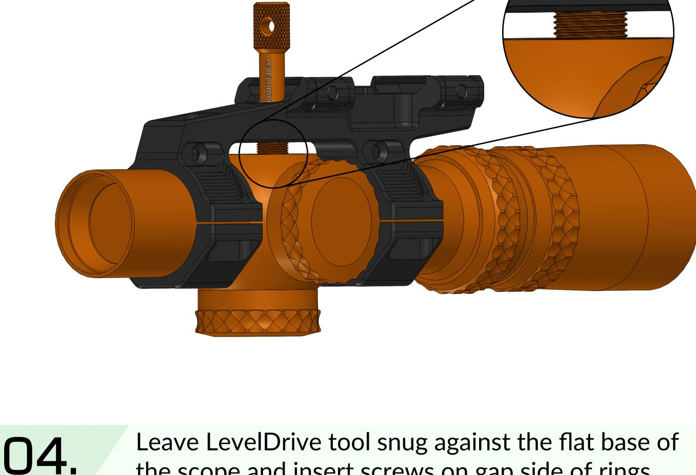
the scope and insert screws on gap side of rings.
