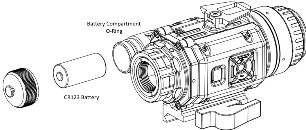
**Figure 3. NOX with Removed Battery Compartment Cover**
