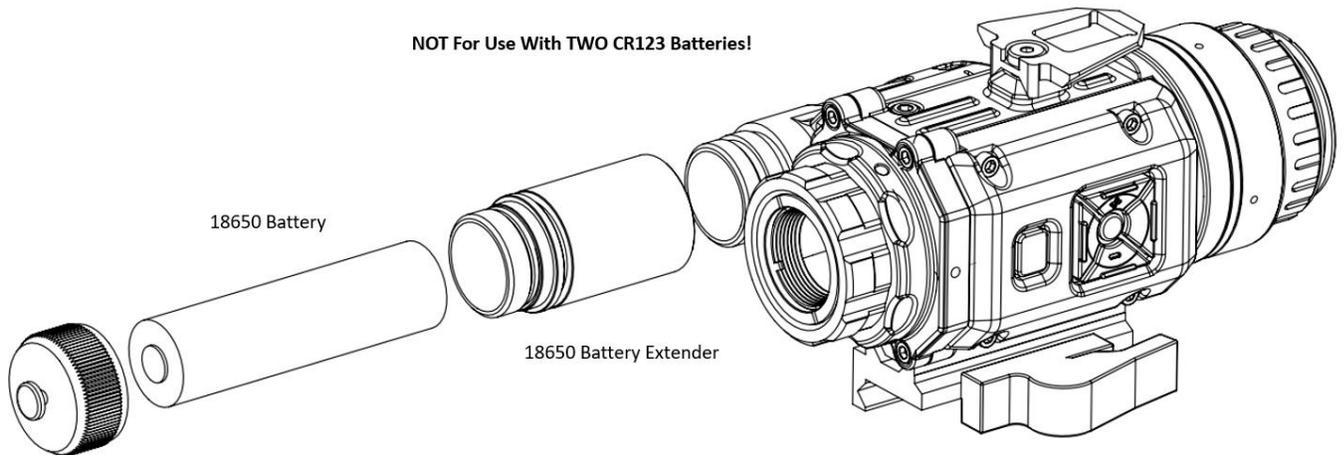
**Figure 4. Installation of the Battery Extender and 18650 Rechargeable Battery**
