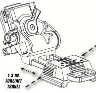
Simultaneously depress both buttons allowing the carriage to move forward or aft. Release buttons to lock.
