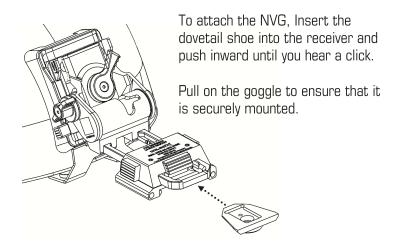
To detach the NVG, hold the NVG then depress NVG release button, then pull outward.
