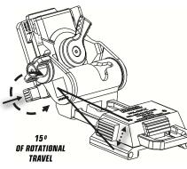
Rotate tilt angle adjustment knob CW to raise angle or CCW to lower the angle.
