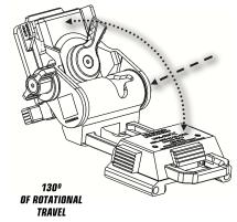
Depress flip release button and position carriage in stowed or operational position. Release button to lock in place.
