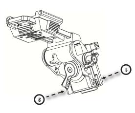
To lock the mount permanently to the Shroud, press lever (1) inward. To unlock the mount to enable the breakaway feature, push the lever (2) inward.
