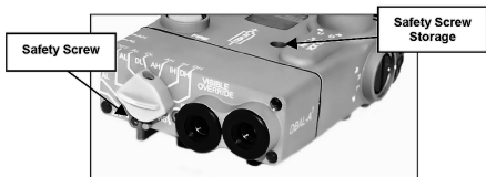
Figure 3-3 Safety Screw Installed (shown in Training Mode)
