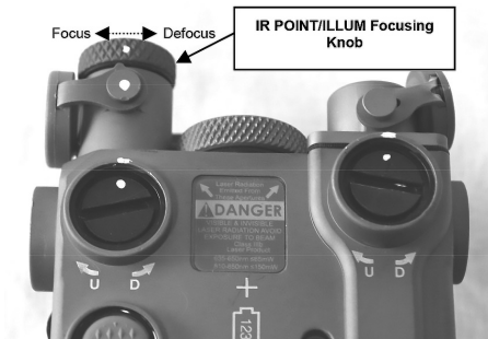
Figure 3-10 The IR POINT/ILLUM Focusing Knob
