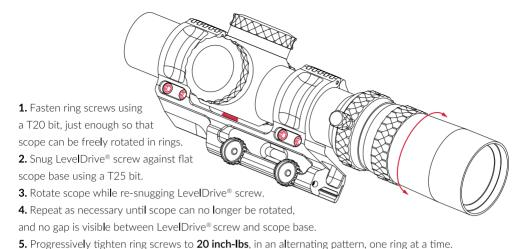
A FIXED TORQUE DRIVER, OR ONE WITH A NARROWER ADJUSTMENT RANGE, IS MORE ACCURATE. PRO TIP
